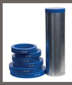
Mounting tools are necessary to mount bearings, bushings, sealing rings and pulleys safely, precisely, damage-free and quickly. Especially when mechanically mounting bearings, it is crucial that the bearing is supported on the inside and outside to avoid damage that leads to premature bearing damage.
